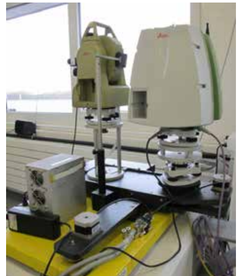
Figure 18: Tilt calibration station for the Leica ScanStation C10. The tilt sensor as it is mounted in the scanner is also observed over temperature.
