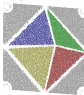
Figure 27: Derived objects, such as building corners, are located within the scan data separately for each face of the scan and compared against the location of the corner found by the Leica TS30. The plates are built and measured in advance of mounting so the relationship between the total station prisms and the corner is known in advance.
