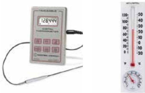
Figure 6: The traceable thermometer on the left is far more expensive than the Acurite® thermometer on the right, whose uncertainty is not explicitly given.
