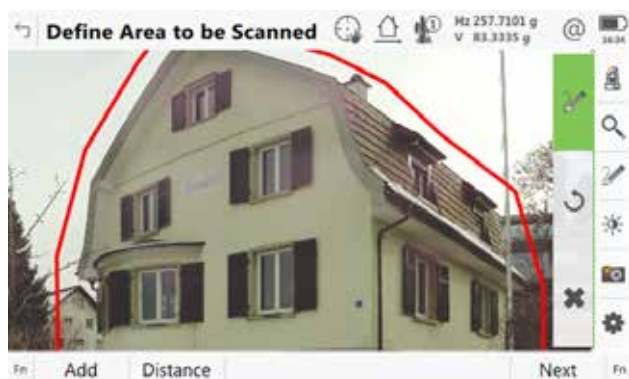
Figure 10 – Live video stream with polygonal scan area definition.
