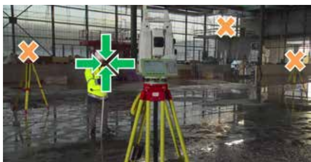
Figure 5 – Using the PowerSearch filter to ignore non-relevant targets.
